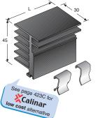
High power dissipation, extruded heatsinks designed to accommodate one or more TO218/TO247 packages via a clip retaining feature (clips available separately). Shaped to minimise board space, with a threaded slot provided to aid assembly. Choice of thermal resistance.
