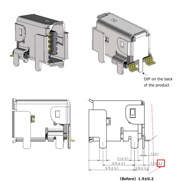
After the change, all products will be inspected by location checkers in the assembly process to prevent defective products from escaping.
